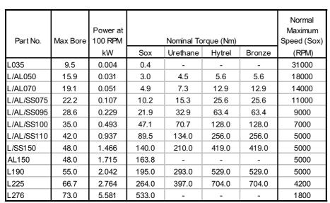
Power at 100 RPM based on Sox only.
